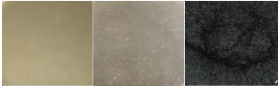
Figure 7. Digital photograph of (a) liquid PCM mixture, (b) gel PCM (c) Thermal enhanced PCM with the addition of nanomaterials
