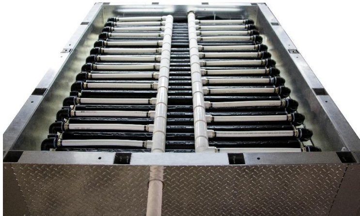
Figure 11. Top sectional view of heat-exchange header and manifold
